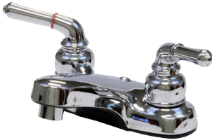
912409 LL423014-C-LF 4" Center Set Lavatory Faucet Zinc Die-Cast Spout Metal Lever Handles Ceramic Disc Cartridge With 50-50 Pop-up 1/2" IPS Connections
